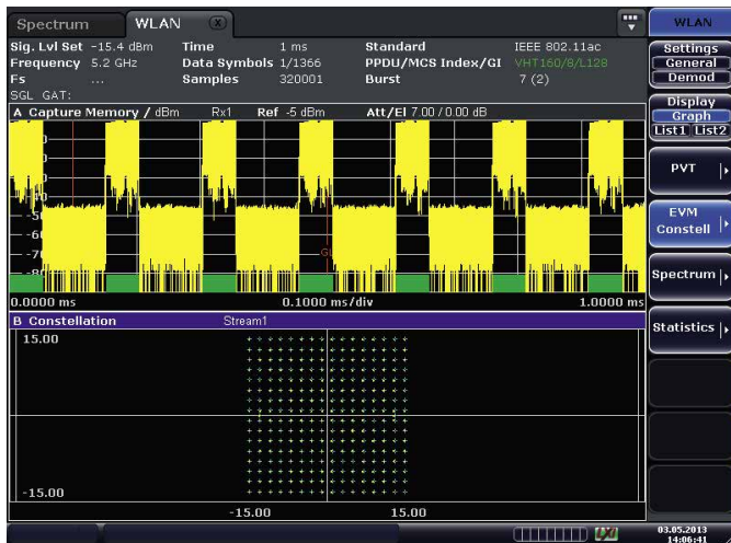
Fig. 2 The upper diagram shows seven demodulated WLAN bursts. The constellation diagram of a 256QAM is shown at the bottom. The clear constellation point matrix indicates high signal quality. Any deviations from this pattern provide useful information about the error source.
