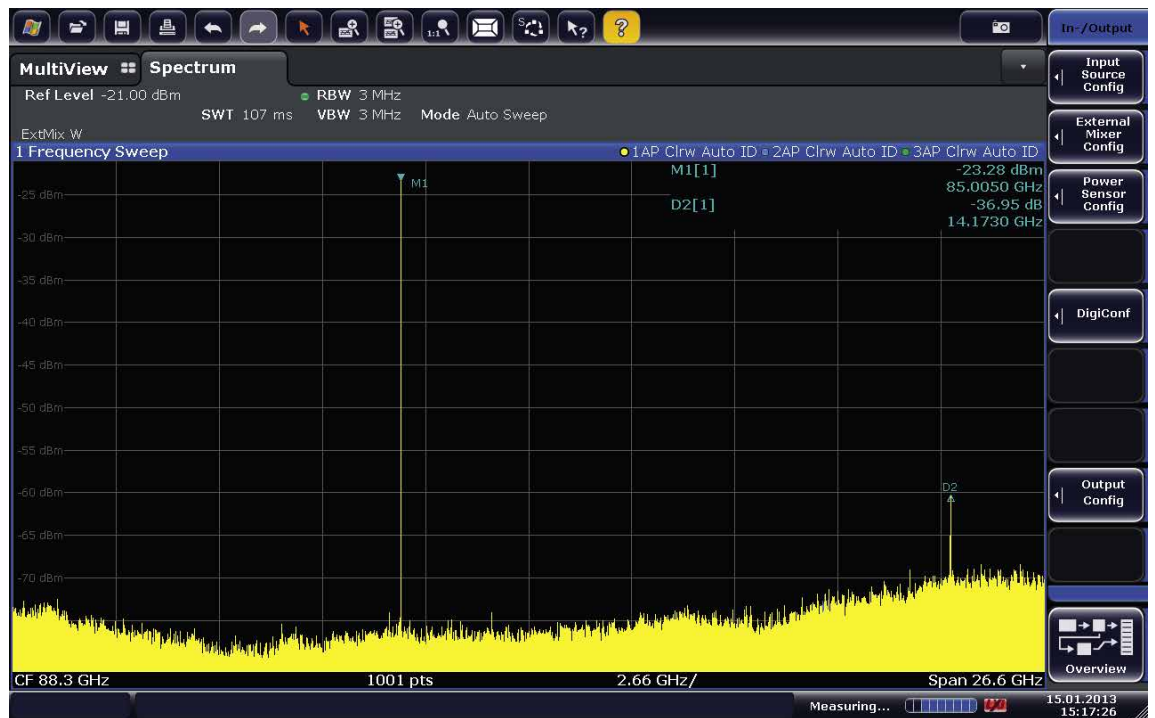
Fig. 6 The built-in signal identification function detects and suppresses multiple response signals so that only the signal of interest is displayed.
