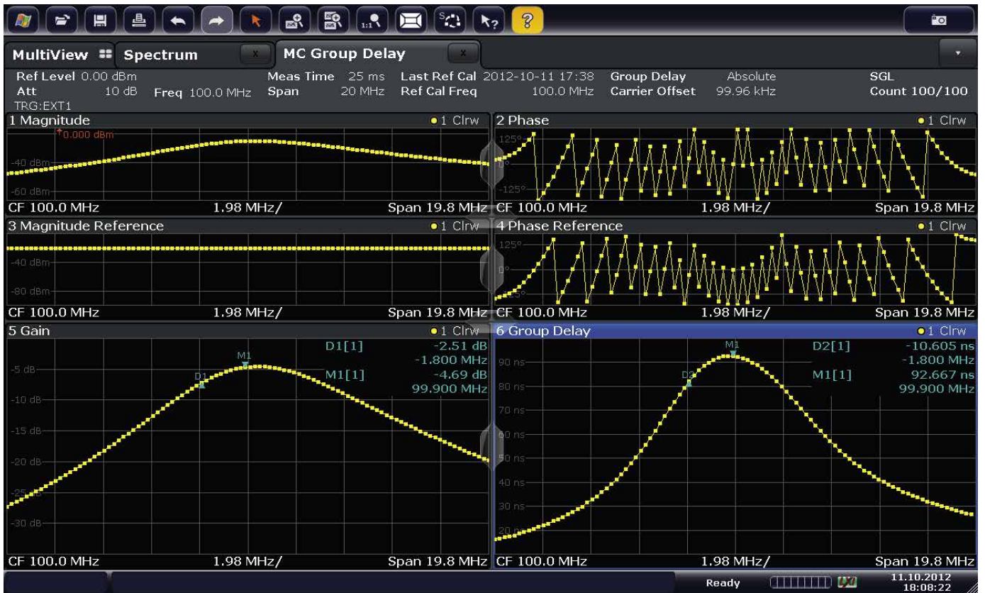
Fig. 4 Nice and clear: Example of DUT measurement with bandpass characteristic. The user can see the amplitude and the phase of the applied multi-carrier signal (windows 1 and 2). Apart from this signal, which is present at the DUT output, the reference signals from the calibration measurement can be displayed at any time (windows 3 and 4). By comparing the reference signal and the measured signal, R&S®FSW-K17 determines the transfer function as a measure of the amplitude distortions (window 5) and the group delay as a measure of the phase distortions (window 6).
