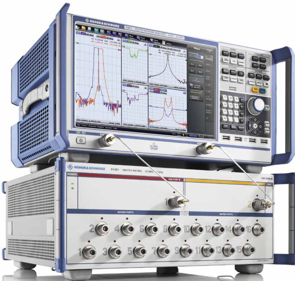
Fig. 1 Multiport network analysis with the R&S®ZNB. Using an R&S®ZV-Z81 model .66 switch matrix provides a total of 16 test ports.
