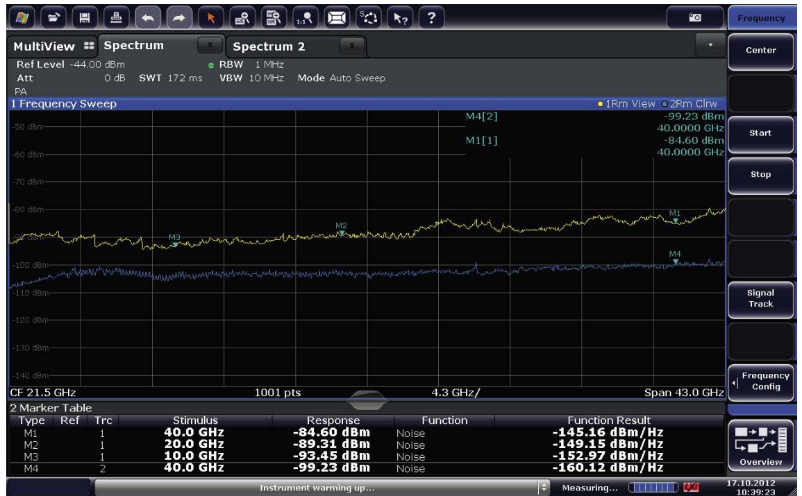
Fig. 2 Displayed average noise level (DANL) of the R&S®FSW43 signal and spectrum analyzer up to 43 GHz with preamplifier off (yellow) and on (blue).
