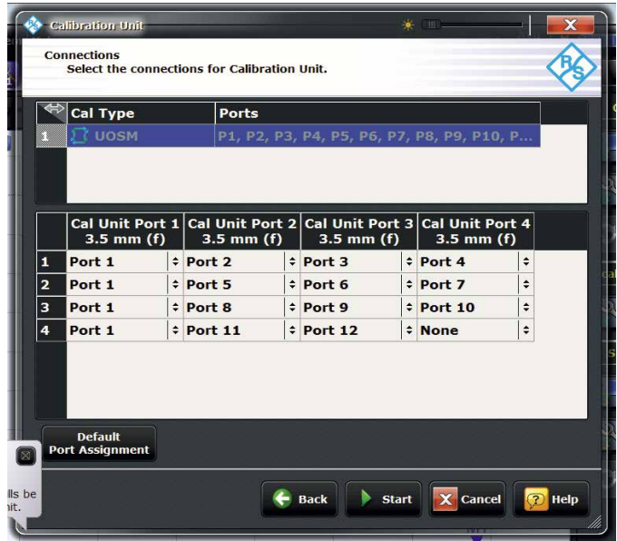
Fig. 6 12-port calibration using a four-port calibration unit.
