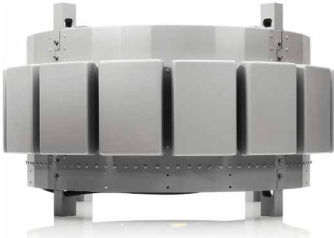
Fig. 3 The R&S®AD016M broadband communications antenna operates in the frequency range from 960 MHz to 1220 MHz and is ideal for applications involving the LINK 16 data radio standard. Due to its stackability, the top of the mast is free for other sensors.
