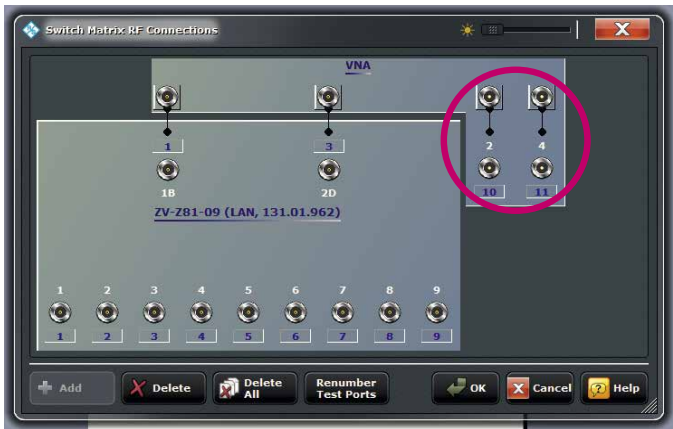
Fig. 4 11-port network analysis system, with two ports on the R&S®ZNB as additional ports.
